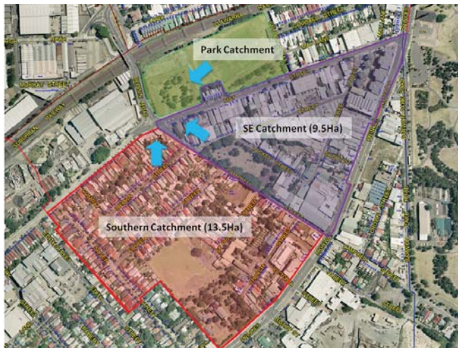
Detention Basin catchment diagram, Storm Consulting
